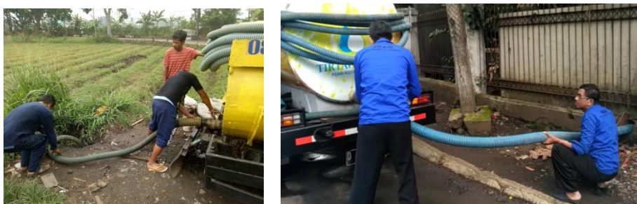
Figure 1. Discharge of collected septage at “dumping points” in Bandung, Indonesia (Source: Author)
