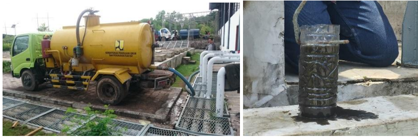
Figure 2. Poor effluent quality of treated septage due to ineffective septage treatment system – Effluent sample taken from a septage treatment plant in Denpasar- Indonesia with a capacity of 400m 3 /day (Source: Author)
